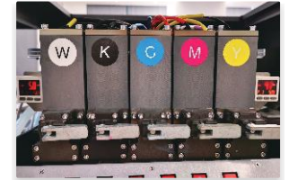
Negative Pressure System
