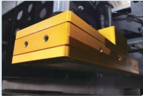
Enhanced water-cooling LED UV lamps cure the ink quickly during high speed printing
