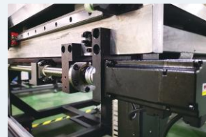
Lead screws driven by dual 400w AC motors for precise Y movement
