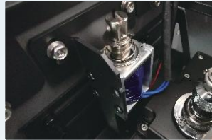
Auto height detector for up to 100 mm thick of material
