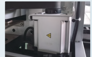
750w AC servo motor assures accurate and durable X movement
