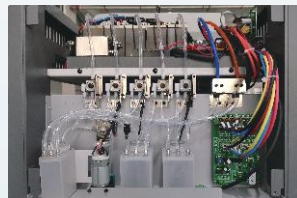
Gntek negative pressure system assures the excellent ink flow and stable jetting
