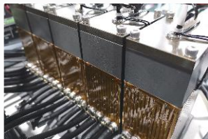
Temp. self-control sub tank system always warms ink flow
